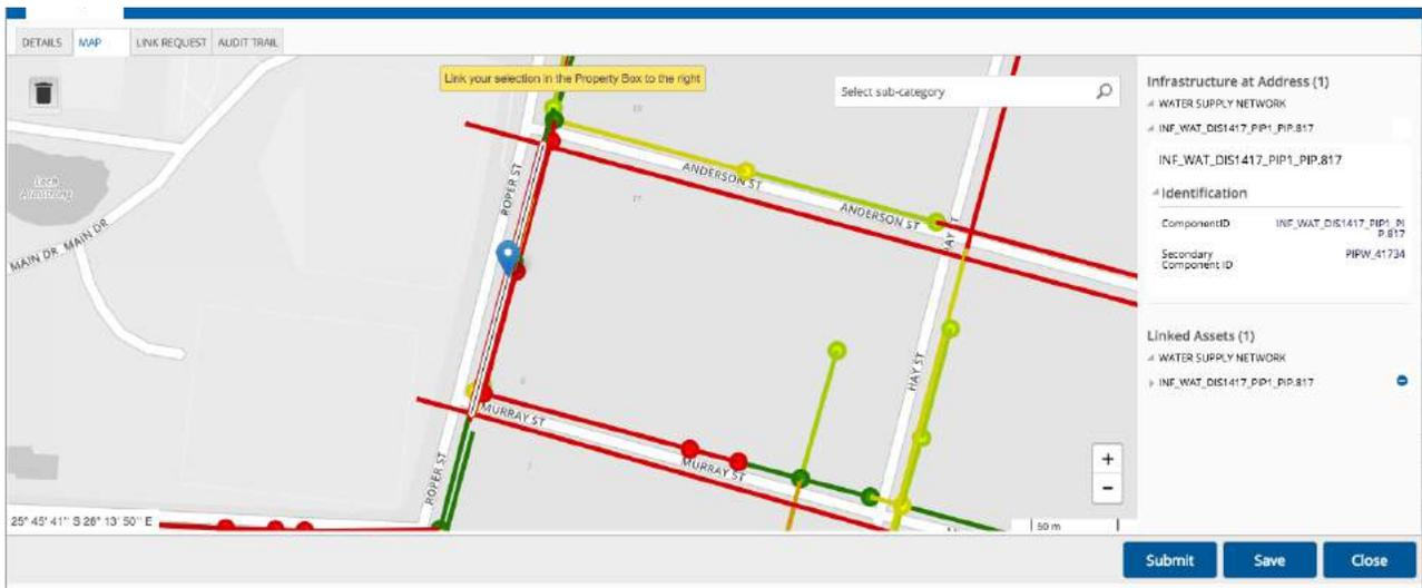
Figure 3: Geographically enabled incident logger
